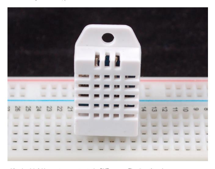
Likewise, it is fairly easy to connect up to the DHT sensors. They have four pins
