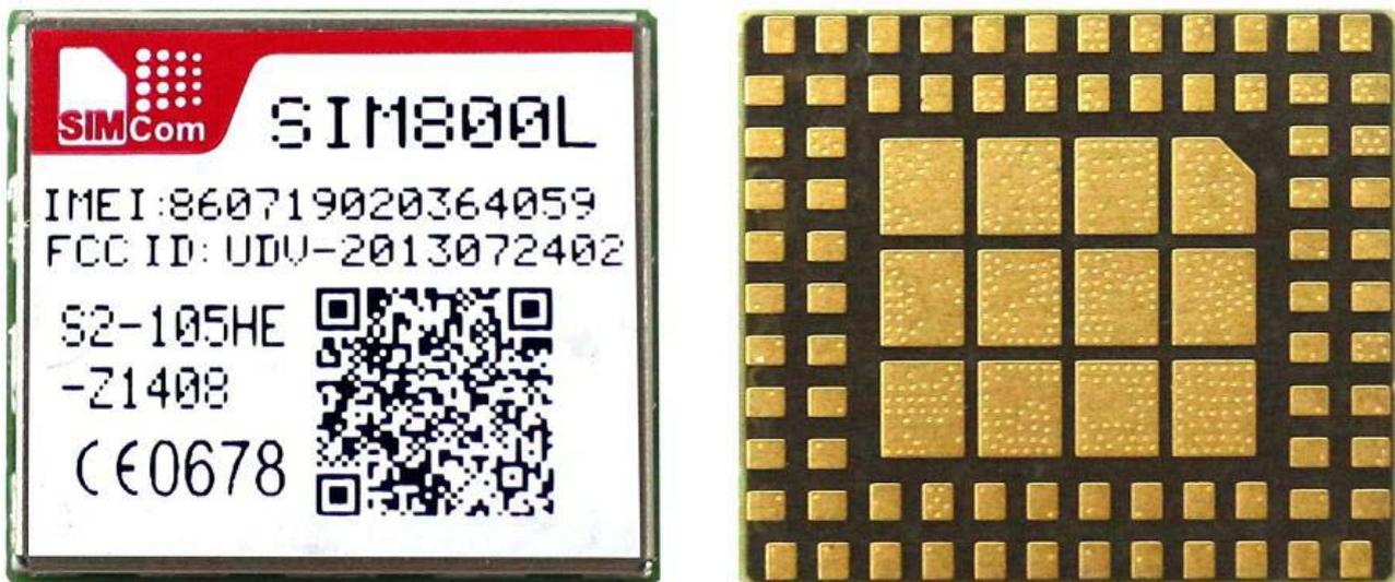
Figure 57: Top and bottom view of SIM800L
