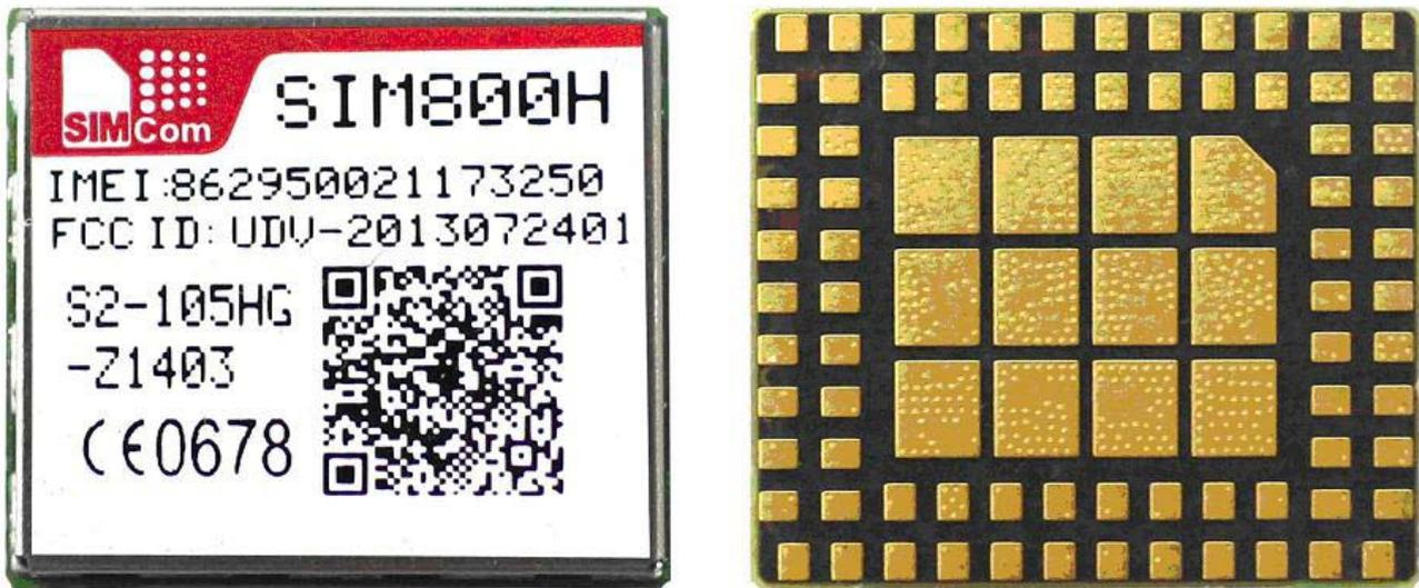
Figure 56: Top and bottom view of SIM800H
